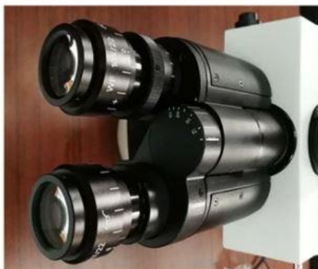
Seidentopf Head, With WF10x/22mm Eyepiece
